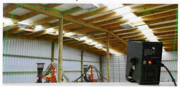
Once mounted in a suitable position plug the laser into a power outlet and position yourself beside, below, or behind the laser. Do not stand in front of the laser.
